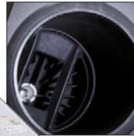
Melt tank with dual pre-melt grids.
