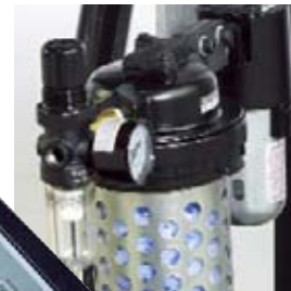
Air-dry modules use standard factory air and replaceable desiccants.
