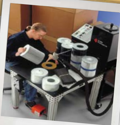
Foot Switch Activated, Timed Shot Automatic Application
