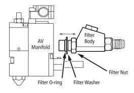
2. Thread the Filter Body into the AV Manifold until tight. Loosen the Filter Body (no more than one turn) to achieve the orientation desired.
