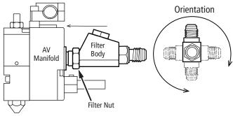
3. Hold the Filter Body in position and tighten the Filter Nut until it rests firmly against the washer. Filter assembly should be tight to the AV Manifold.
