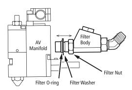
2. Thread the Filter Body into the AV Manifold until tight. Loosen the Filter Body (no more than one turn) to achieve the orientation desired.
