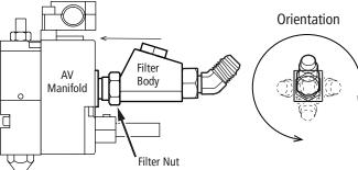
3. Hold the Filter Body in position and tighten the Filter Nut until it rests firmly against the washer. Filter assembly should be tight to the AV Manifold.
