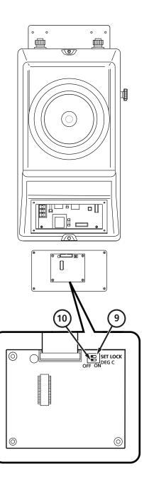
**High Limit:** The exclusive High Limit Feature limits the Set Point for any zone. This limit is adjustable between 250°F and 475°F.
