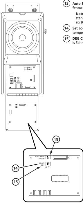
Auto Standby and Auto OFF: Slide dip switch left to turn on feature. Neither, either, or both features can be activated.
