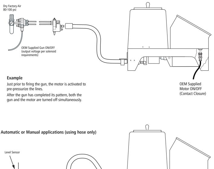
When the hot melt bath drops below the required level, the motor is activated to pump material into the bath.
