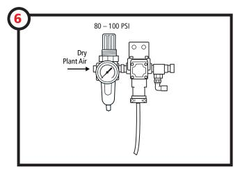
Connect dry plant air to the regulator (6) and adjust to 80–100 psi.
