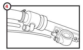
Attach the flexible vacuum hose to the vacuum assembly and connect the airlines to the wand assembly.
