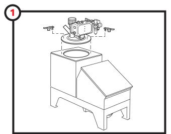
Place the ProFill-S lid assembly on top of the hot melt adhesive tank. Lock the lid in place using the toggle clamps (two provided).
