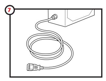
Plug the control box power cable in to the wall (120VAC or 220VAC single phase) or into the adhesive supply unit using the auxiliary power output cable (922-218 for 120VAC or XP-922-218 for 220VAC).
