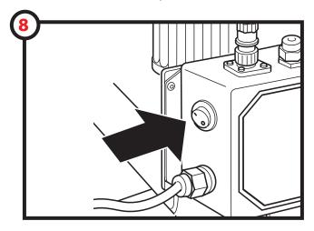
Turn the ProFill-S "ON" and the tank will begin to fill if needed.
