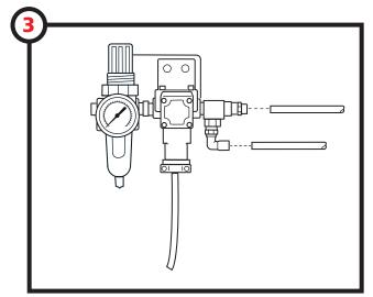
Connect the airlines for the vacuum wand assembly to the ProFill-S air control assembly.
