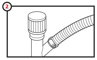
Connect the flexible vacuum hose to the inlet on the tank lid assembly.
