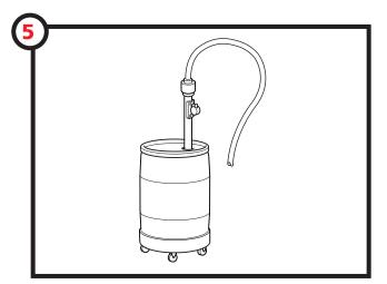
Insert the wand assembly into an auxiliary adhesive storage container. For best performance, do not attach the wand to the container as this can dampen vibrations from the wand assembly.
