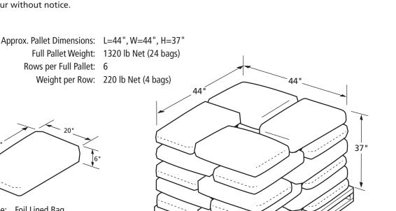
Container Type: Foil Lined Bag Container Dimensions: L=30", W=20", H=6" Container Weight: 55 lb Net
