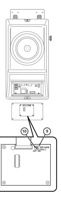
**High Limit:** The exclusive High Limit Feature limits the Set Point for any zone. This limit is adjustable between 250°F and 475°F.
