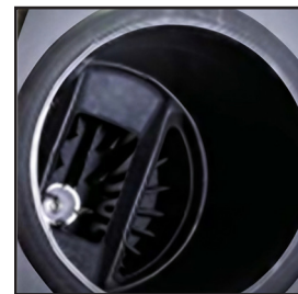
Melt tank with dual pre-melt grids.
